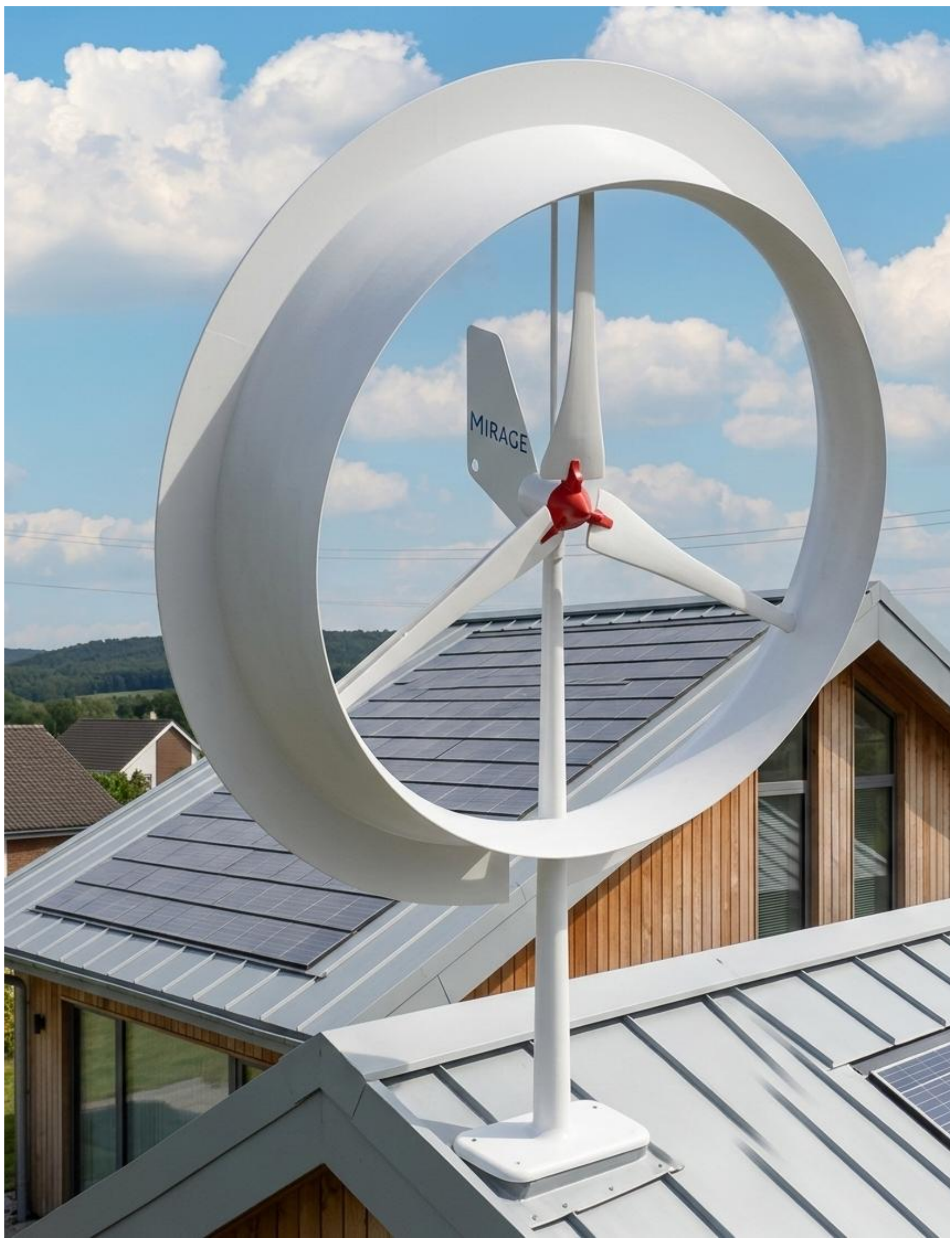
Fully assembled ducted HAWT prototype — rooftop field installation
